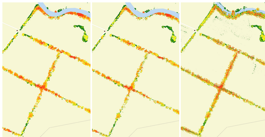
Fig. 5: Canopy height model (CHM) at Westregeln study area using DSM1, iDSM20 and UAV data sets (from left). DSM1, DSM20, DTM source: State Office for Surveying and Geoinformation of Saxony-Anhalt (LVerGeo).
