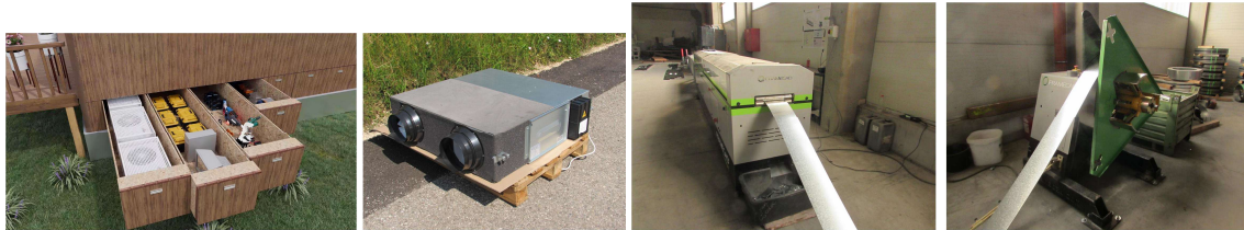
Left 1: drawers instead of basement. Left 2: air ventilation system with heat and humidity recovery. Right 1: This machine can produce the frame of a GEMINI 60 house in 3 hours. Right 2: The steel comes from this coil.
