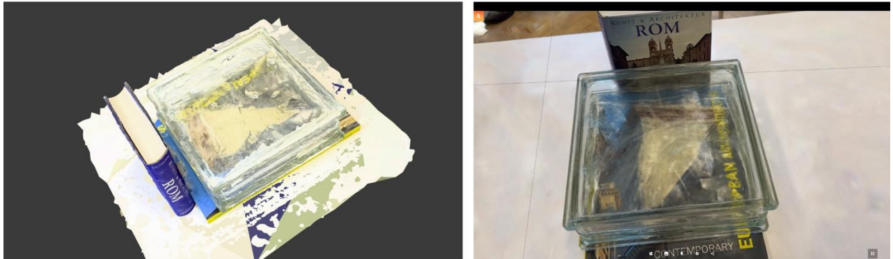
Fig. 2: Scanning a glass brick. Left image, 3d model with photogrammetry; right image, 3d model represented as Gaussian splats.
