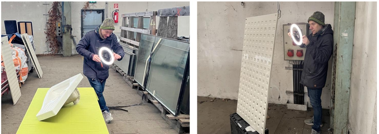
Fig. 4: Offsite scanning of extracted building elements from the stocks of materialnomaden [MATERIALNOMADEN n.d.].
