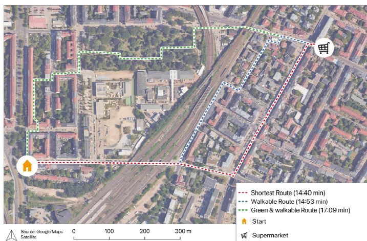
Fig. 3: Implementing hiBike and hiWalk into OpenRouteService (ORS) to generate routes optimised for active mobility rather than just the shortest or fastest paths. Considering walkability and/or bikeability in routing can help quantify how close cities are to being a “15-minute-city for all”.
