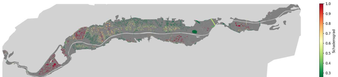
Fig. 7: Estimation of building damage based on the calculated flood height and the digital building models.
