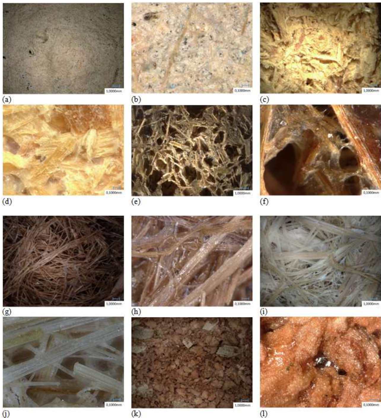
Figure 2. Microscopic images at 20x (left) and 100x (right) magnification with Keyence digital microscope. (a), (b): wastepaper; (c), (d): wood shavings, (e), (f): straw, (g), (h): seaweed, (i), (j): hemp, (k), (l): cork bark
