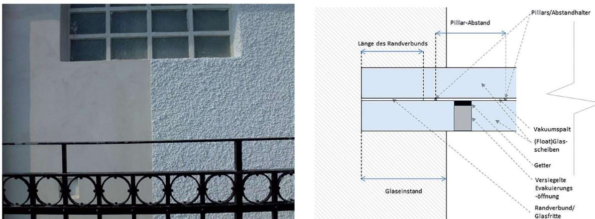
Fig. 6: Aerogel-plaster test surfaces (Image by the Author), fig. 7: Schematic Constituents of vacuum glazing products (Image by the Author)
