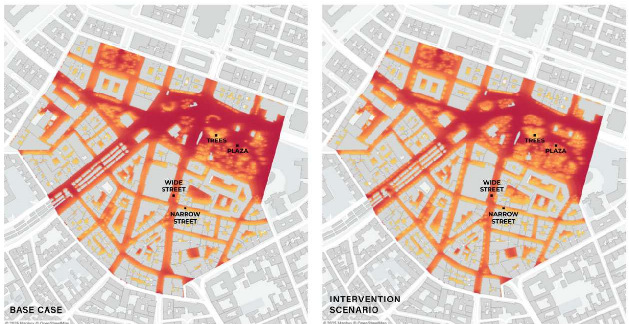
Fig. 2: Two microclimate simulations carried out for a highly frequented central urban location in Vienna, Austria: (left) the current state; (right) the urban interventions. The predefined locations, from which the temporal daily heat profiles are extracted, are marked within the target area.
