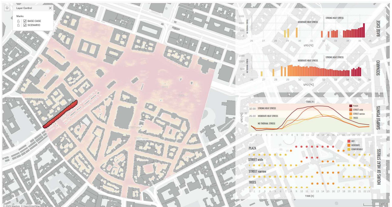
Fig. 5: Demonstration of the interconnected visualizations, where selecting areas of strong heat stress on the map triggered instantaneous updates in the histogram view, allowing a side-by-side comparison of the base case and intervention scenario.
