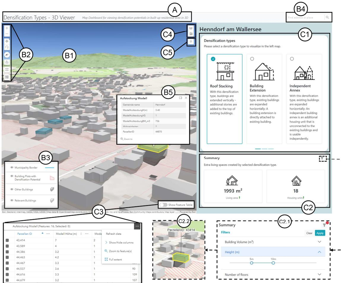
Fig. 3: User Interface: Use case in Henndorf am Wallersee. Densification type ‘roof stacking’ is selected. (A) header, (B1) map view, (B2) map controls, (B3) layer list, (B4) address search panel, (B5) pop-up window, (C1) densification type selection cards, (C2) summary panel, (C2.1) expanded filter with user-defined height threshold, (C2.2) simulated roof stacking model selected by filter (C3) feature table, (C4) measurement toggle, (C5) daylight and shadow simulation widget.
