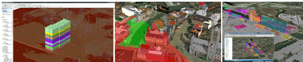
Fig. 22: 3D-GIS attributes with information of volumes, Fig. 23: visibility research, Fig. 24: Spatial structure and destination maps
