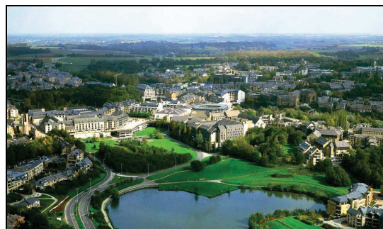
III. 14. (To be added) Louvain-la-Neuve university town: all storm water is led to a reservoir which appears to be a lake, which saves infrastructure costs and attracts housing investment.
