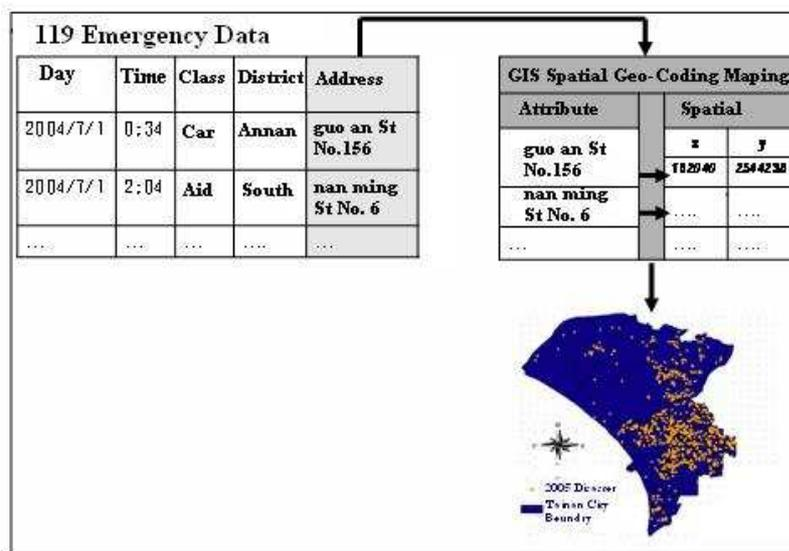
Fig 1 Illustration of coordinate conversion of disaster locations
