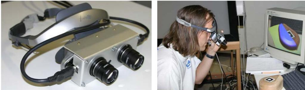
Abb. 1: Augmented Reality HMD Cy-Visor. [Quelle: HLRS, 2003]
