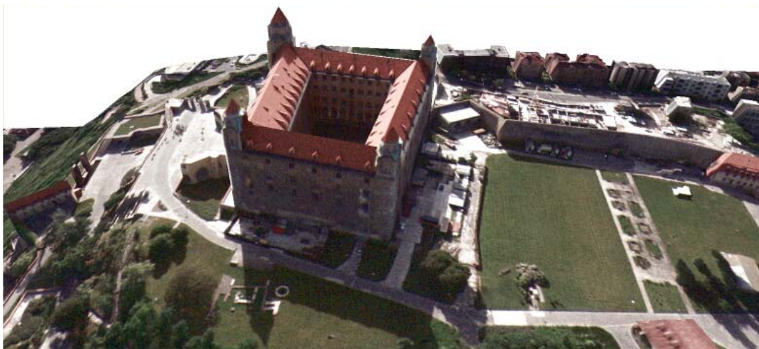
Figure 6: Semiautomatic texture mapping was used on the DTM and the castle model input shown in the Figure 8. Source texture is an aerophoto taken from about 2100 meters above the terrain.
